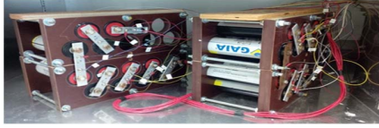
Fig. 4. 24 cell GAIA battery pack.
